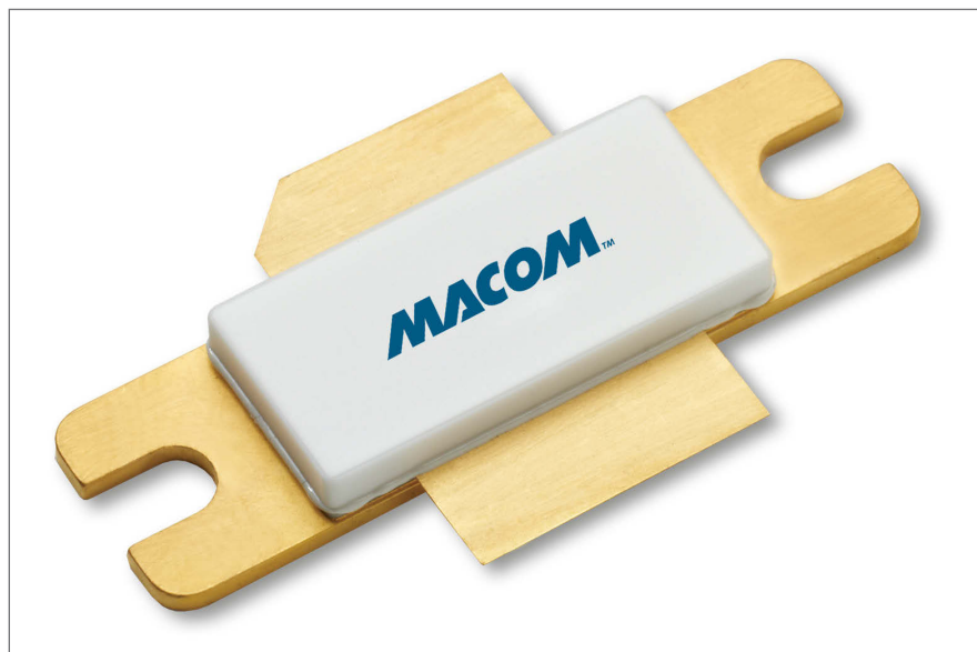
Figure 1 | The gallium nitride on silicon carbide (GaN on SiC) pulsed power transistor for military and civilian radar pulsed applications offers designers a typical 17 W of peak output power with 63 percent efficiency.
