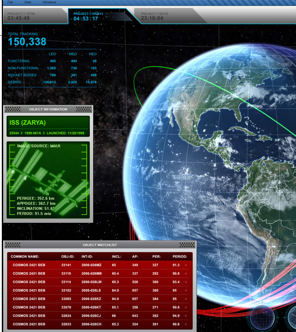
Space Fence is a fully digital S-band radar system that can track debris as small as 10 centimeters. Photo courtesy of Lockheed Martin.
