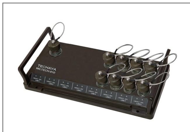
Figure 4 | The Techaya MILTECH 910 is a rugged, 8-port Power over Ethernet (PoE) gigabit switch. Photo courtesy of MilSource.
