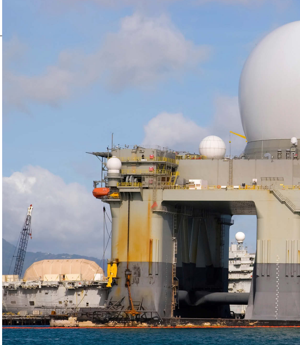
The SBX-1 is a floating, self-propelled AESA radar station that is able to move to areas where it is needed for enhanced missile defense. Part of the Department of Defense's Ballistic Missile Defense System, the SBX-1 has as its primary task discrimination/identification of enemy warheads from decoys, followed by precision tracking of identified warheads. The floating radar station – mounted on a twin-hulled semi-submersible drilling rig – measures 279 feet (85 meters) from its keel to the top of its radar dome. (Photo courtesy of MACOM and U.S. Department of Defense/Missile Defense Agency.)
