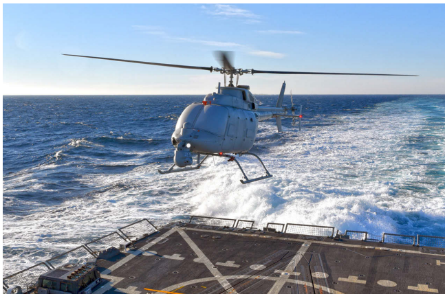
Figure 1 | The MQ8-C Fire Scout unmanned helicopter prepares for landing on the USS Jason Dunham. Photo courtesy of Northrop Grumman.
