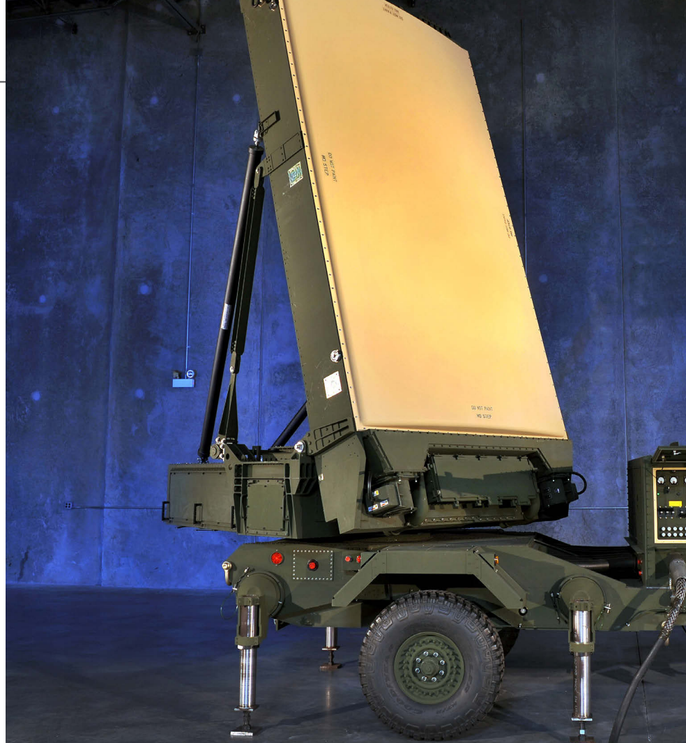
The U.S. Marine Corps AN/TPS-80 G/ATOR system uses Northrop Grumman's Active Electronically Scanned Array (AESA) radar technology. Photo courtesy of Northrop Grumman.
